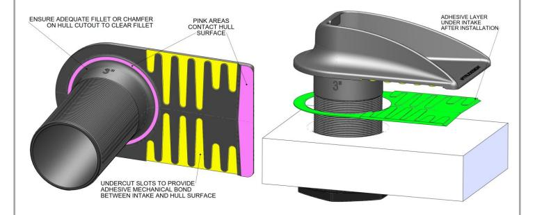
In the case of adhesive sealants tighten the nut down onto the washer ensuring it is hand tight. Check the Strainer is flat against the outside of the hull, and both contact points are made. After 1 day of hardening, tighten a further ¼ turn or to a maximum of 15 Ft Lbs. There is no need to over-tighten the Nut.
